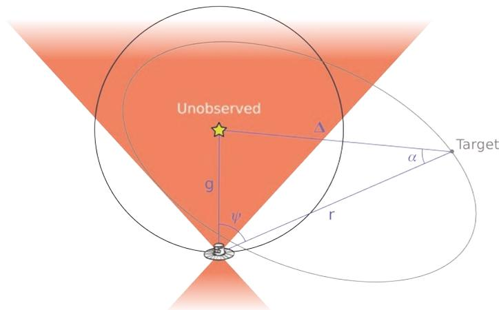
Fig. 2: Gaia observing geometry. Knowing Gaia and the target heliocentric distances ( $g$  and  $\Delta$ ) and the solar elongation ( $\psi$ ) of the observation, the target-Gaia distance ( $r$ ) and phase angle ( $\alpha$ ) are easily computed.
