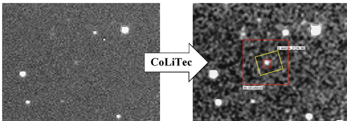
**Fig. 2:** One of the well-known results of the CoLiTec software. The detected and discovered object, the Comet C/2012 S1 (ISON), having an image size of 5 pixels, has been shifted by 3 pixels on a set of four CCD frames.
