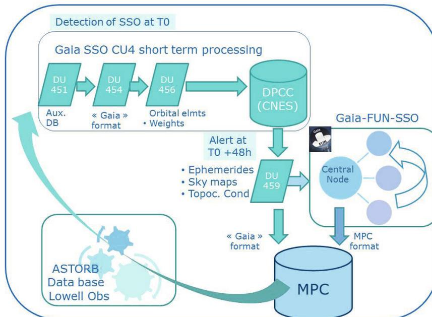
**Fig. 1:** Data flow of the Gaia short term data processing, involving the Gaia-FUN-SSO observation, their processing by the Minor Planet Center and the updating of the Gaia auxiliary data through the ASTORB database.
