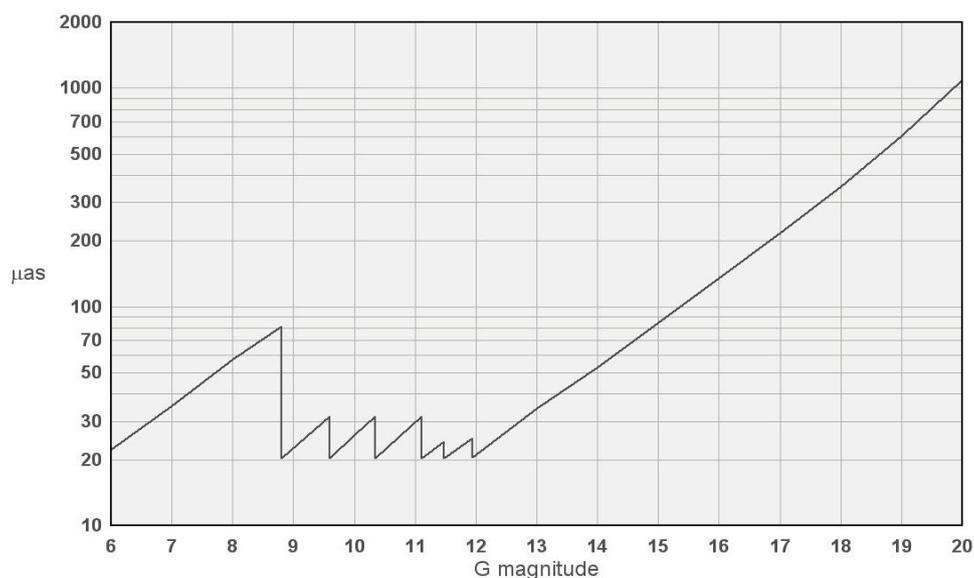
Figure 1. Single-transit accuracy for a point-like stellar source, as a function of apparent brightness. The G magnitude is the “Gaia” spectral response (unfiltered in the visible, for AF CCDs), a proxy of V.
