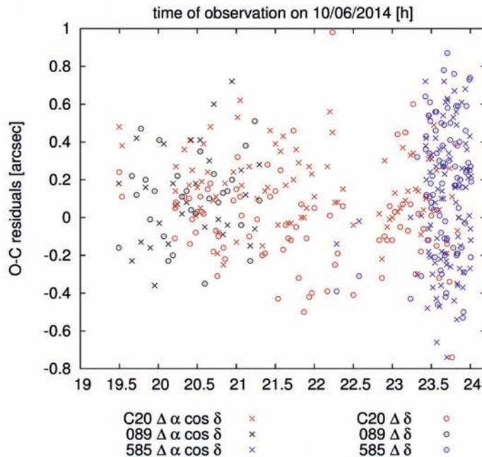
**Fig. 3:** Residuals in the astrometric measurements performed during the triangulation campaign of the NEO 2014 HQ<sub>124</sub>. Observatories are color coded, whereas the residuals for the astrometric angles are denoted by circles and crosses, respectively.
