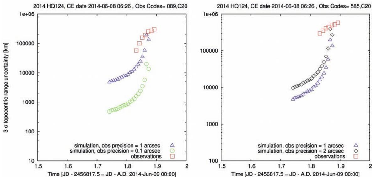
**Fig. 4:** A comparison between simulated and actual triangulation observation results. The graphs show the remaining topocentric positioning uncertainty of 2014 HQ<sub>124</sub> for triangulation based ranging measurements at specific times. Left : Triangulation was performed with observations by 089 and C20. Right : Only observations by 585 and C20 were considered. A cut-off below 20 degrees of telescope elevation was considered for the simulations.
