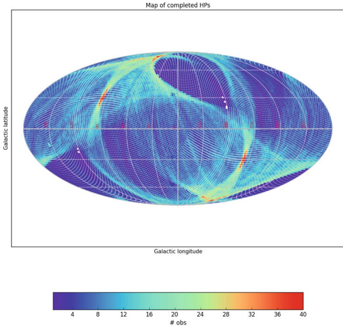
**Fig.3.** Map of the sky covered by Gaia in November 2014. The colour-coding indicates number of individual visits in a given part of the sky. The Ecliptic Poles observed intensively in June/July 2014 are clearly visible. In November 2014 the entire sky was observed at least once by Gaia, allowing for more unambiguous detections of new sources.
