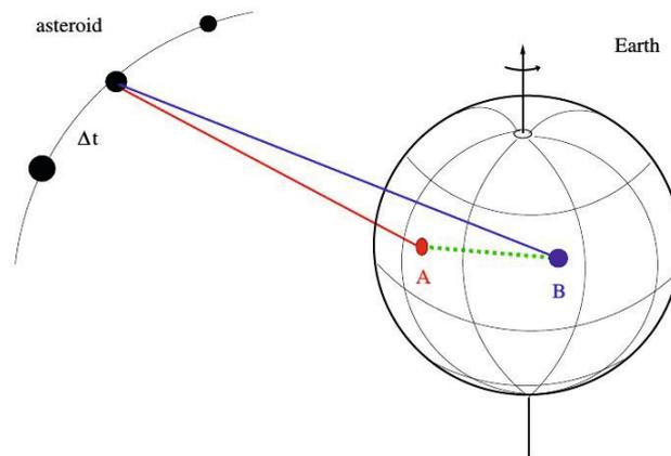
**Fig. 1:** Simultaneous observations of an asteroid by two Earth-bound observers. The dotted green line corresponds to the baseline between the observing stations. Simultaneous observations can be used to perform optical ranging of a NEO during its flyby.
