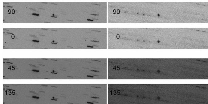
**Fig. 1:** TFOSC-WP image of 4 polarized beams at  $0^\circ$ ,  $45^\circ$ ,  $90^\circ$  and  $135^\circ$  separated by 60 arcsec of NEA 276049, V-band. Right is single 120 exposure image, left is result of combining of 5 images using median filtering.
